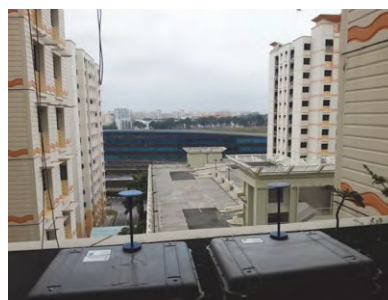
Figure 1. Co-located DustTrak Monitors inside Environmental Enclosures (Model 8535) in Singapore
